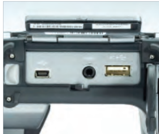
From left to right: USB mini for PC image download, NTSC video, USB-A for memory stick image transfer
