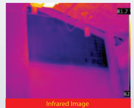
Fusion Image Showing Missing Insulation
